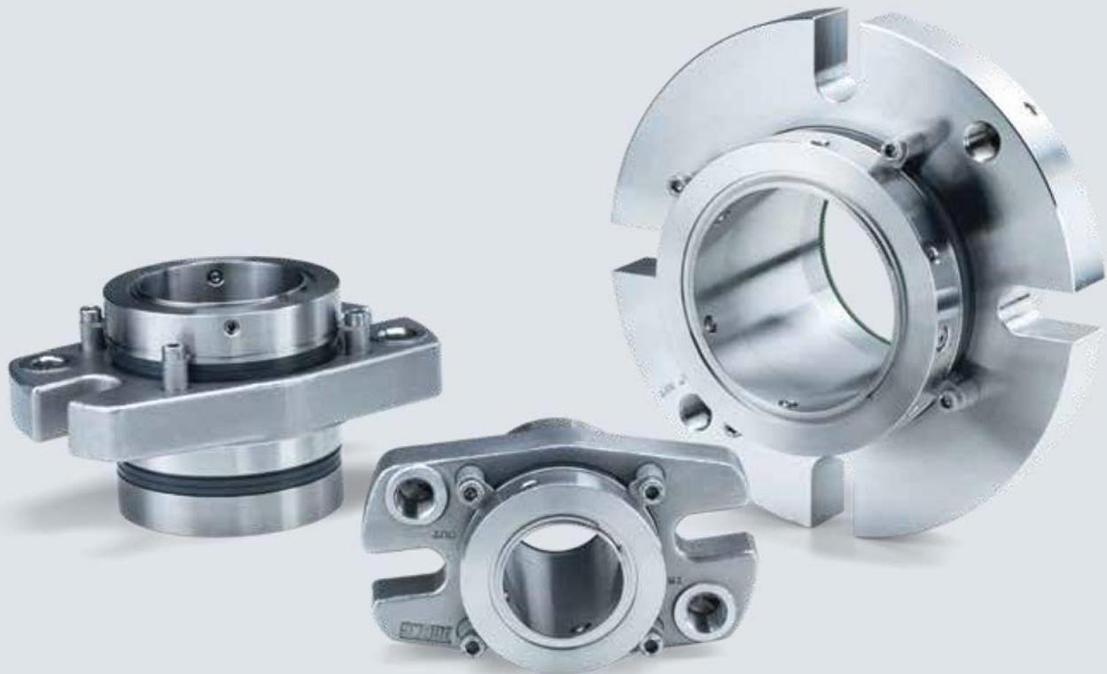
The DEPAC mechanical seal type 322 is a stationary, tandem-active double-cartridge mechanical seal with integrated barrier fluid pumping assistance. The double pressure relief of the seal faces on the product side also ensures that the seal faces do not open in case of pressure reversal - and that the pressure relief for reducing the friction values is present under all pressure conditions.
